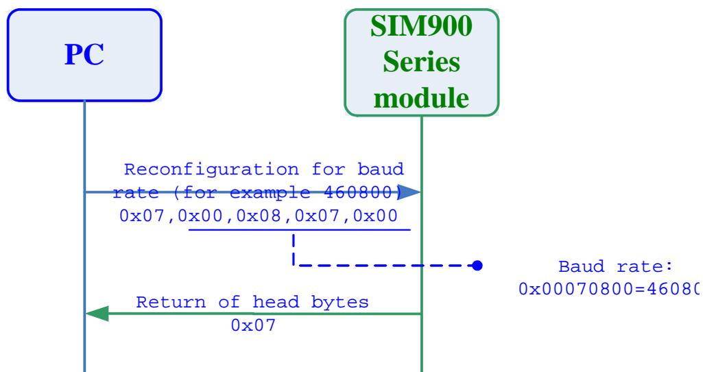
**Diagram 2-5 Reconfiguration for downloaded serial port's Baud rate**
