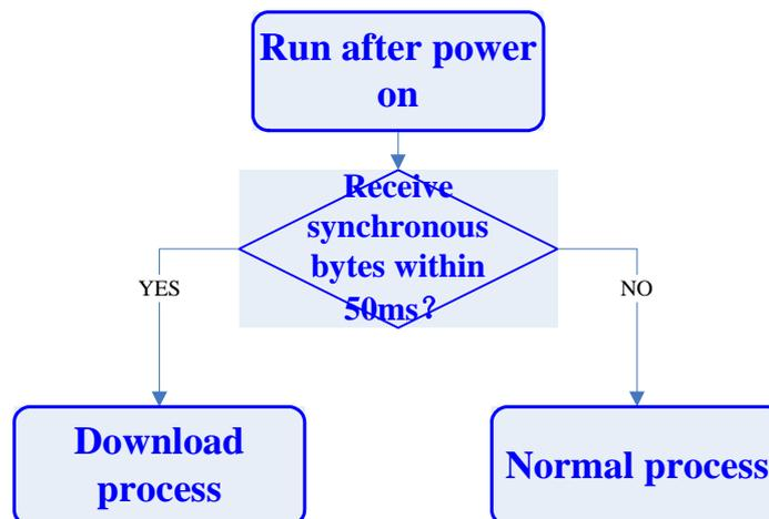
**Diagram 2-2 Process of waiting for synchronous bytes**
