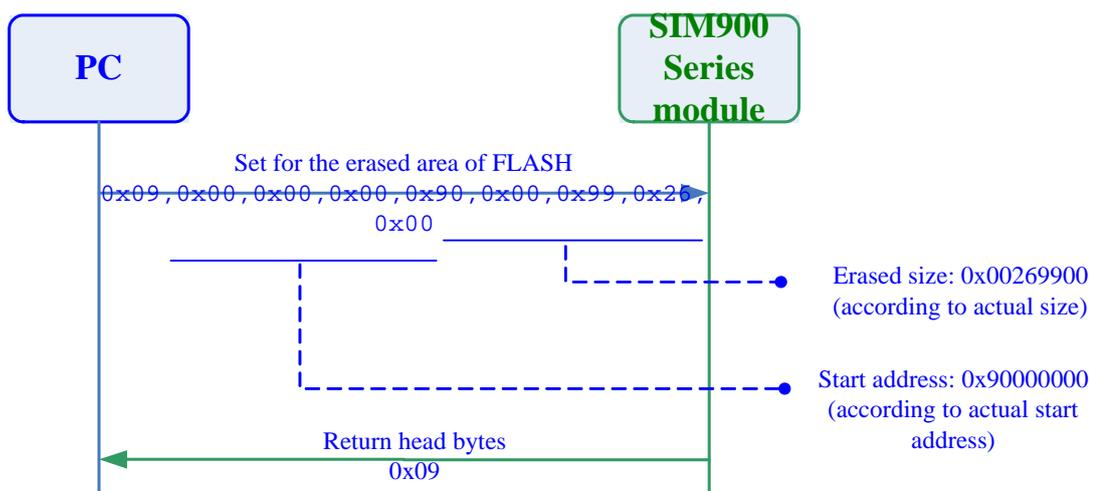
Diagram 2-9 Configuration for erased area of FLASH
