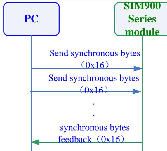
**Diagram 2-3 Detection for synchronous bytes**
